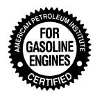
This symbol means that the oil has been certified by the American Petroleum Institute (API). The manufacture only recommends API Certified engine oils that requirements meet the DaimlerChrysler Material Standard MS-6395. Use Mopar or an equivalent oil meeting the specifi-
